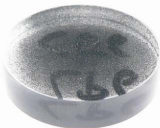
fig 4. Closely-packed monolayer polished section of final concentrate; diameter = 2.5 cm.
