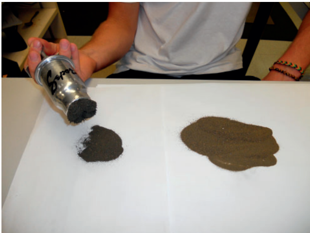
Fig. 8. A hand magnet is commonly used to remove the ferromagnetic fraction (black sand on left) from the heavy mineral concentrate prior to indicator mineral picking (photograph courtesy of Overburden Drilling Management Ltd).
