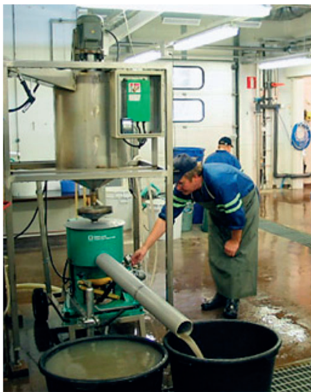
Fig. 5. Lab-based Knelson concentrator used to prepare a preconcentrate for recovery of kimberlite indicator minerals by the Geological Survey of Finland (photo provided by M. Lehtonen, Geological Survey of Finland).
