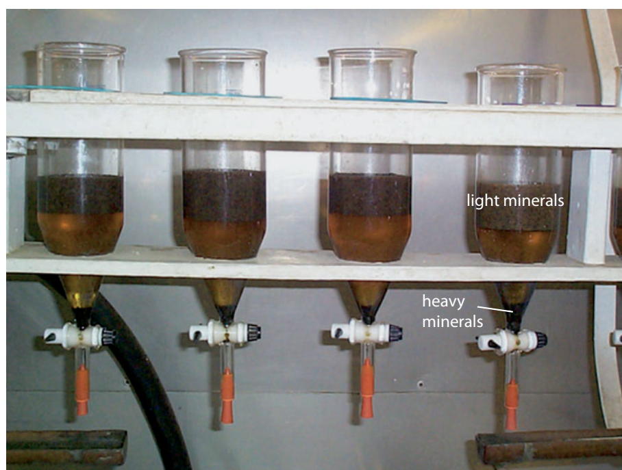
Fig. 7. Separation of heavy and light minerals is carried out using a specific heavy liquid of known density in separatory funnels, Heavy mineral sink and light mineral float to the top (photo provided by Overburden Drilling Management Ltd).
