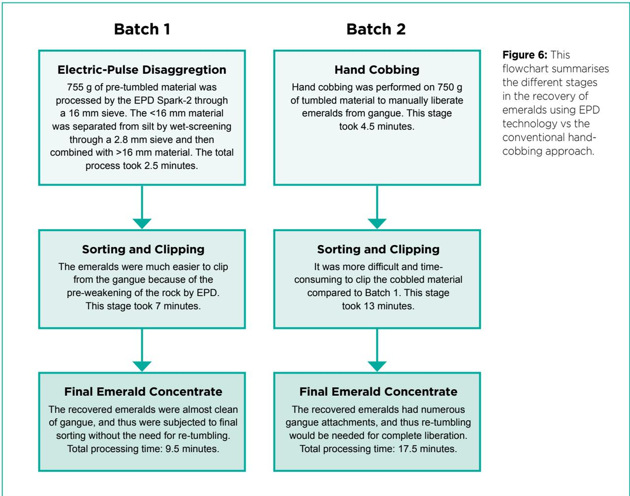
**Figure 6:** This flowchart summarises the different stages in the recovery of emeralds using EPD technology vs the conventional hand-cobbing approach.
