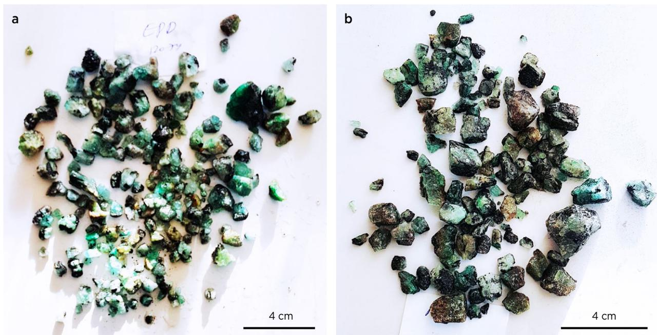
**Figure 10:** These photos show the final emerald concentrates recovered (a) after EPD processing and (b) after conventional hand cobbing. The EPD-liberated emeralds have very little residual micaceous schist material compared to those obtained by hand cobbing. Photos by V. Rudashevsky and O. Alikin.
