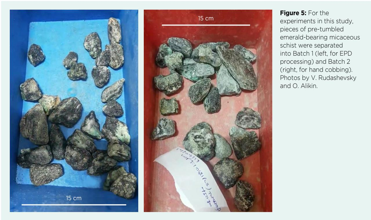
**Figure 5:** For the experiments in this study, pieces of pre-tumbled emerald-bearing micaceous schist were separated into Batch 1 (left, for EPD processing) and Batch 2 (right, for hand cobbing). Photos by V. Rudashevsky and O. Alikin.
