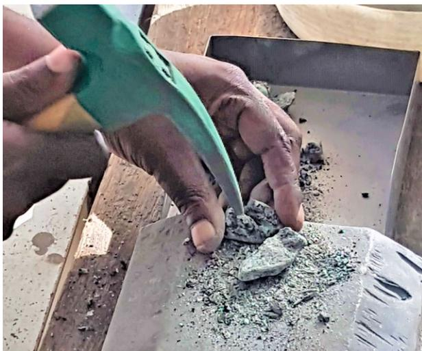
**Figure 7:** Conventional hand cobbing is accomplished using a hammer in order to recover emeralds from micaceous schist. Photo by V. Rudashevsky and O. Alikin.
